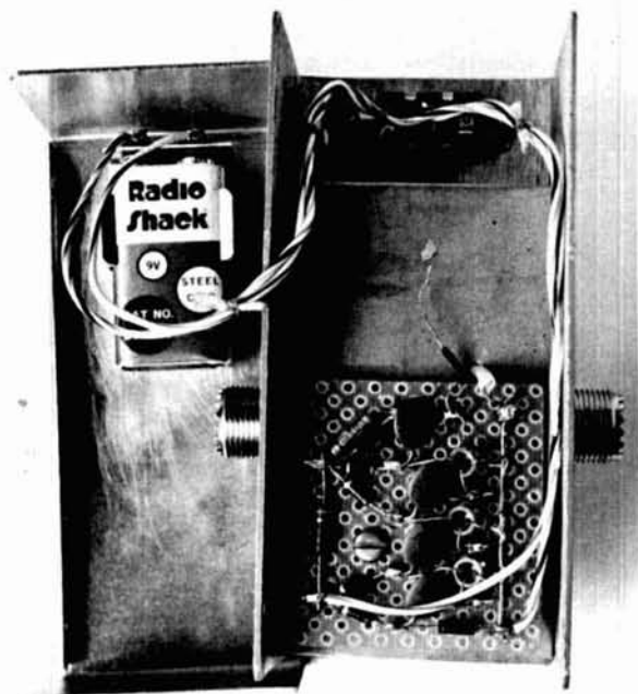
fig. 7. Interior layout of the improved noise bridge is shown in this photograph. A copper electrostatic shield encloses the bridge section. The three leads from the bridge section can be seen at the upper right-hand corner of the perf board. One is a ground lead and the other two are leads from the primary of the toroid. One primary lead is connected to the amplifier output; the other is left unattached as explained in the text.
